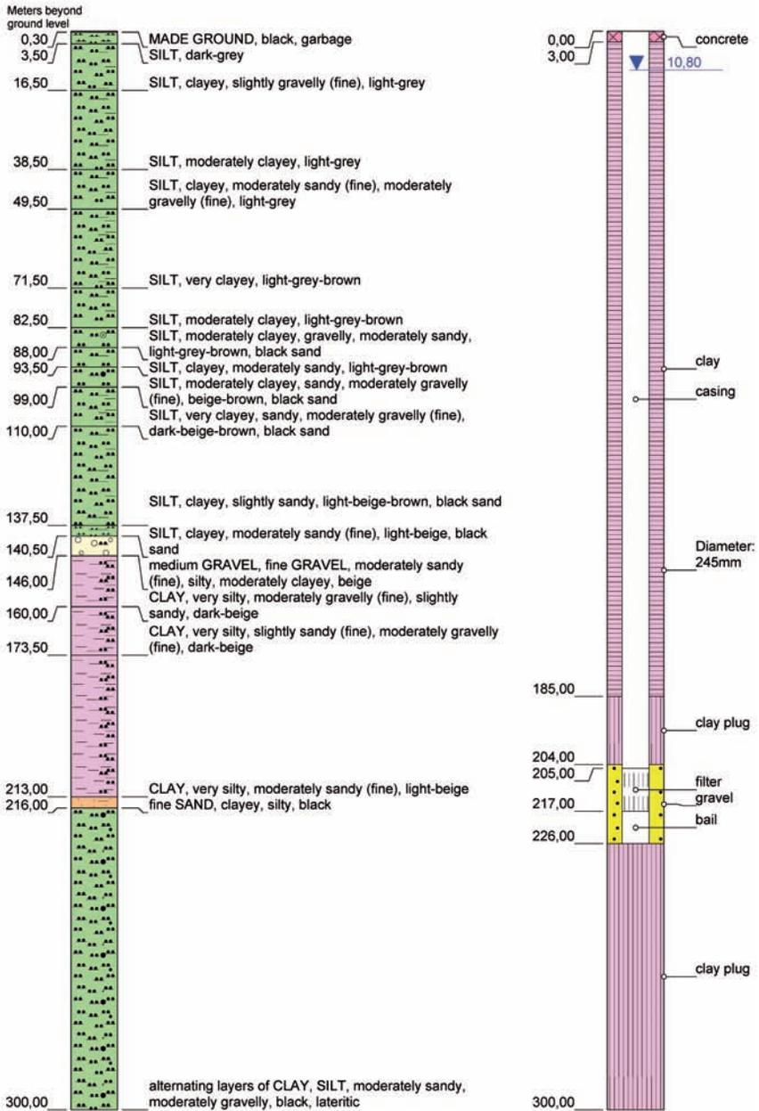
Fig. 10. Geological profile, well building and first results of a pump test in Rier.
