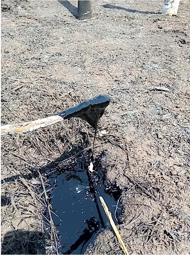
Figure 31: This photograph shows a crack in the surface with an expanse of some 30 cm x 40 cm. This has enabled the emergence of a puddle of oil. Its surface is some 10 cms below the edge of the surface. This photograph gives rise to the conclusion that the oil in this area at least was not removed and disposed of, but, rather, simply covered with earth. A “rod test” shows that the liquid’s viscosity is that of oil.
