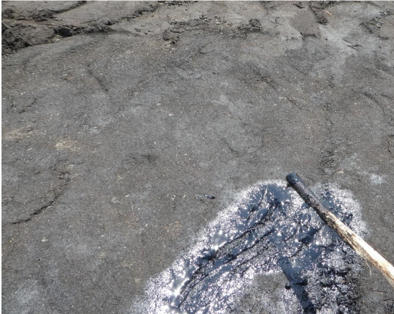
Figure 33: This close-up of the ground shows that oil has risen to the surface. The use of a “rod test” reveals that the liquid’s viscosity is that of oil.
