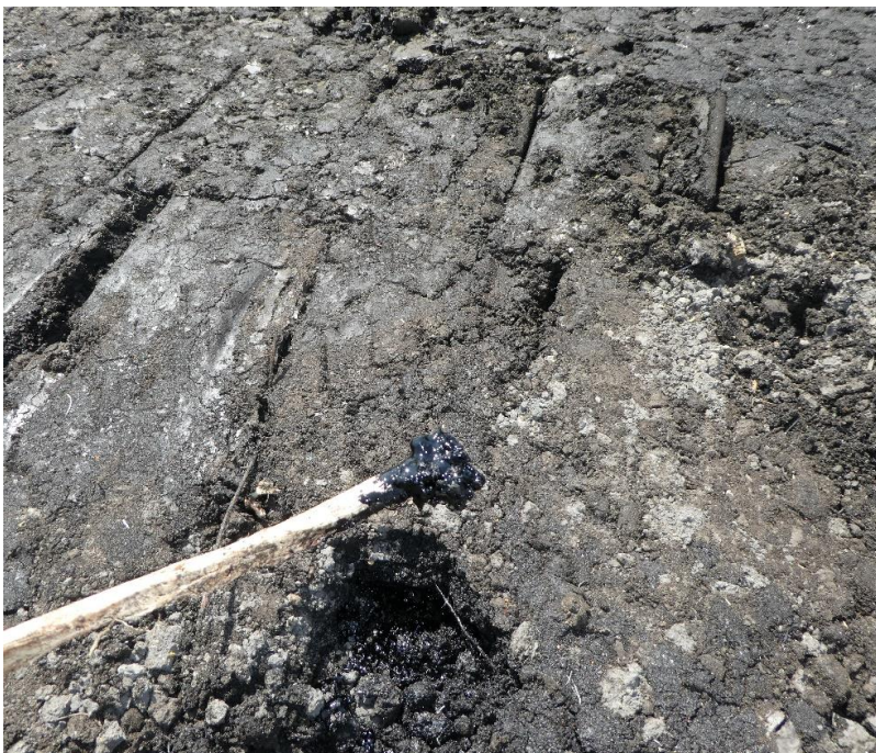
Figure 34: Breaking through the top of the ground with a rod shows that oil and oil saturated earth is to be found some 5 cms below the surface.
